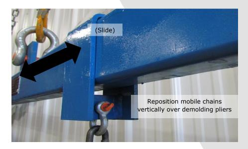
5. Hoist concrete panels to desired location and repeat the procedure for all other concrete panels requiring demolding.
